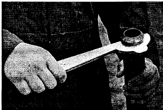
Figure 4.6. Tighten MC Cutting Shoe with MC Combination Wrench.
